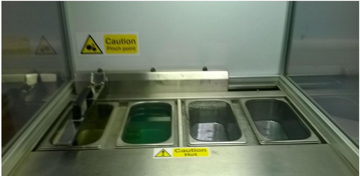
Fig.7 - 4 stage 'Optimal' substrate bath; ultrasonic, lye, post clean and drainage
